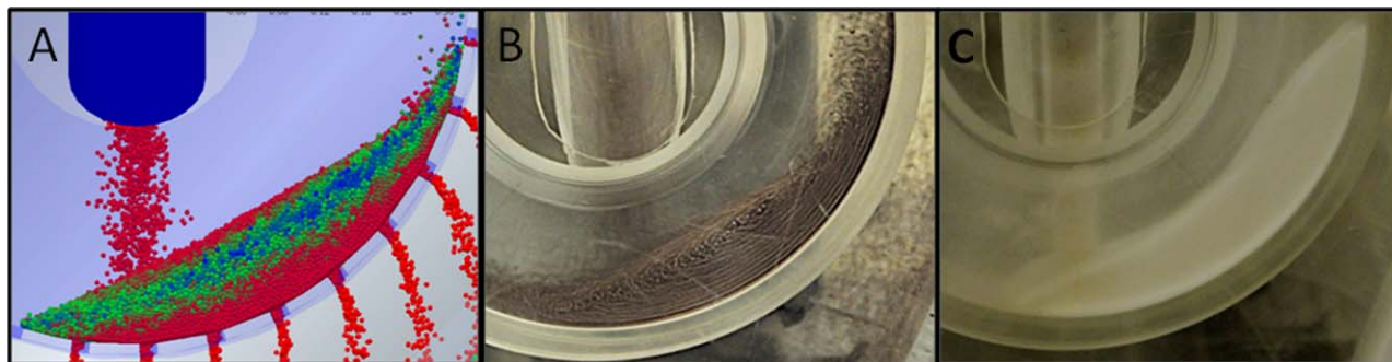
Figure 6. Simulation and validation using lactose and glass beads at 70 RPM.
